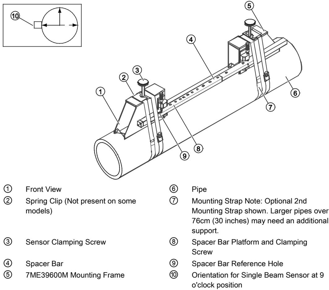
Figure 5-8 Sensor Installation
