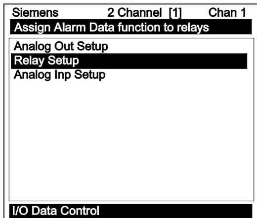
3. To access the [Relay Setup] option list press <Right Arrow>.
