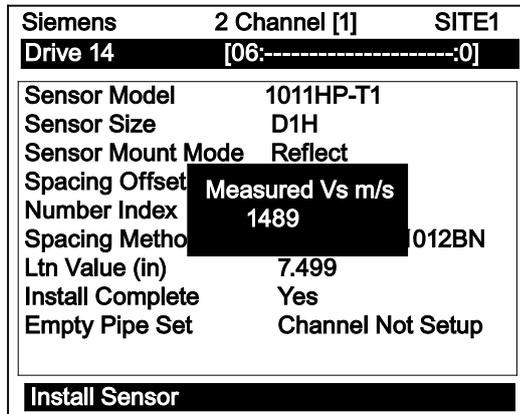
4. Observe the Measured Vs window and verify a correct sound velocity measurement (if known).
