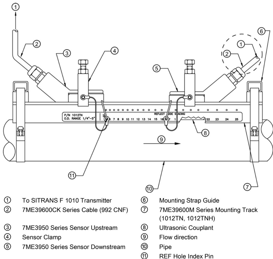
Figure 5-12 Reflect Mount with Model 1012TN Mounting Track (Side View)
