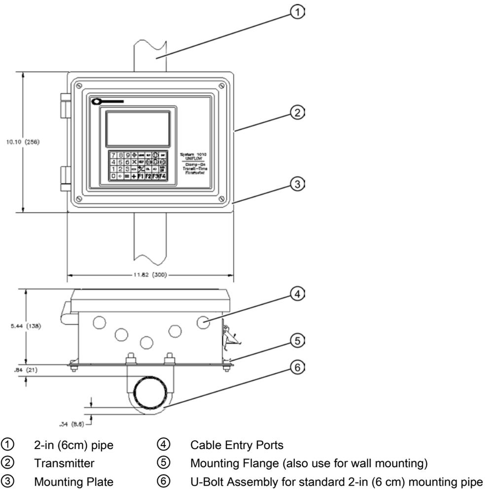
Figure 4-1 Pipe Mounting and Mounting Locations for Transmitter
