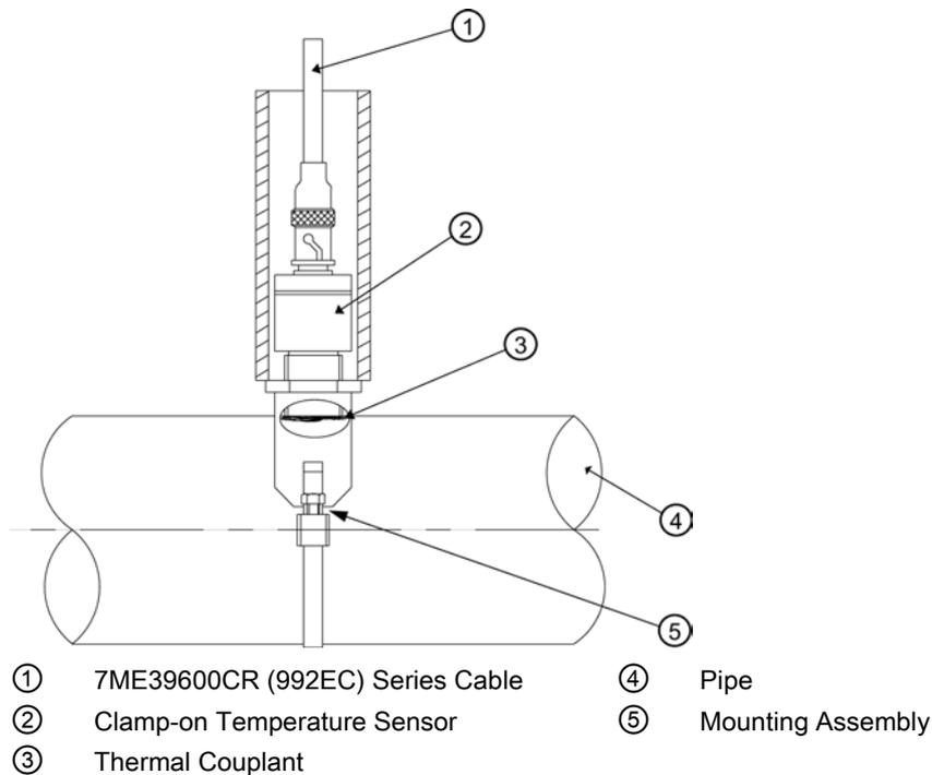
Figure 5-16 Clamp-on Temperature Sensor
