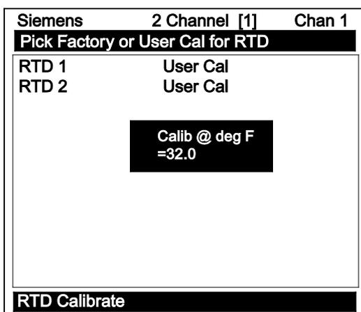
5. To enable numeric entry press the <Right Arrow>, then type in the reading of the reference thermometer (e.g. 72.0).
