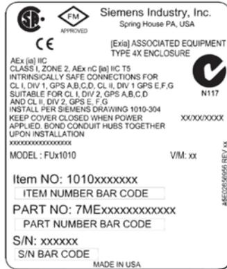
Figure 3-1 Typical Transmitter Label
