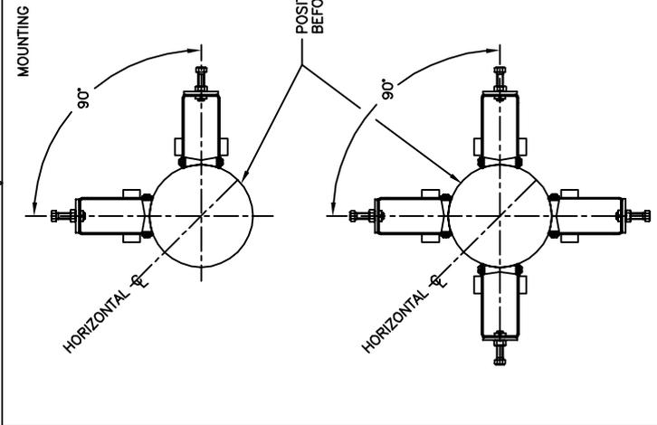
RECOMMENDED INSTALLATION ON HORIZONTAL PIPES
