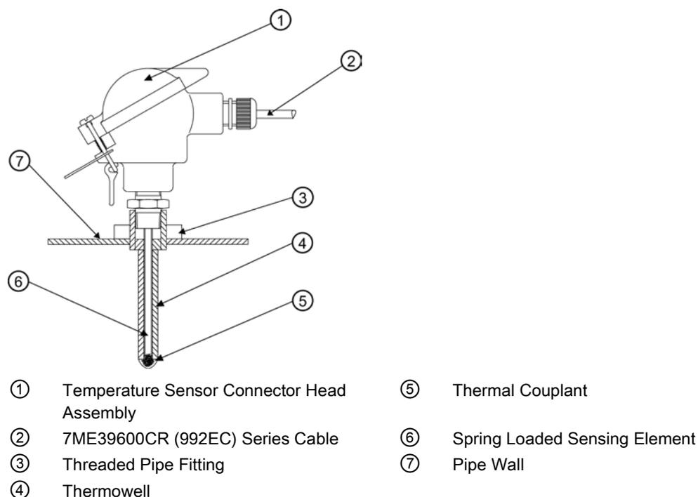
Figure 5-17 Insert Temperature Sensor
