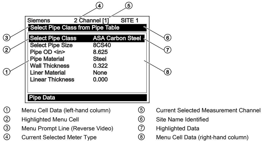
Figure 6-1 Typical Installation Menu Screen
