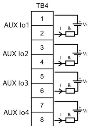
Vc: 24 VDC typical (+15VDC to 30VDC max) Loop Supply
