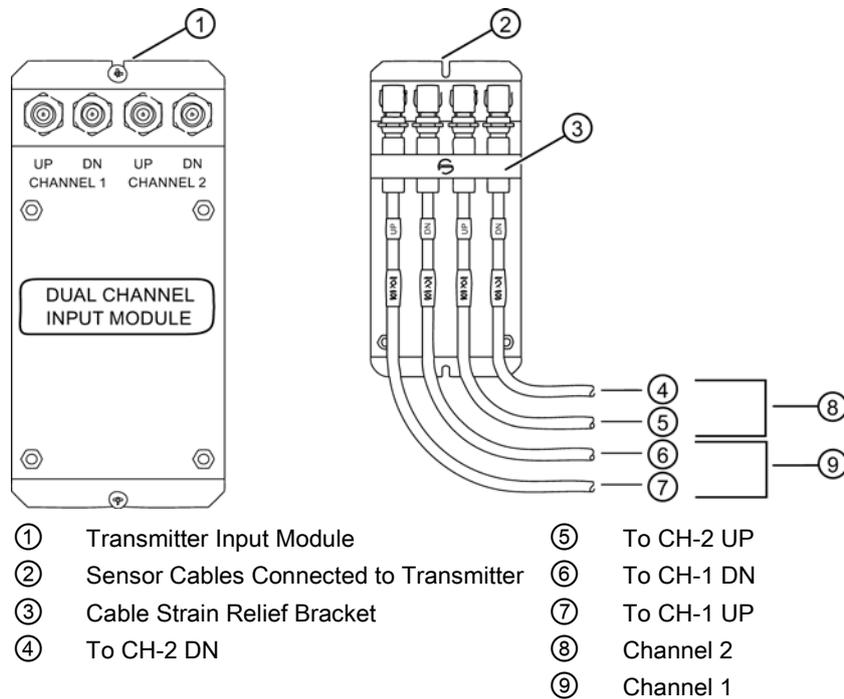
Figure 5-18 Sensor Cable Connections
